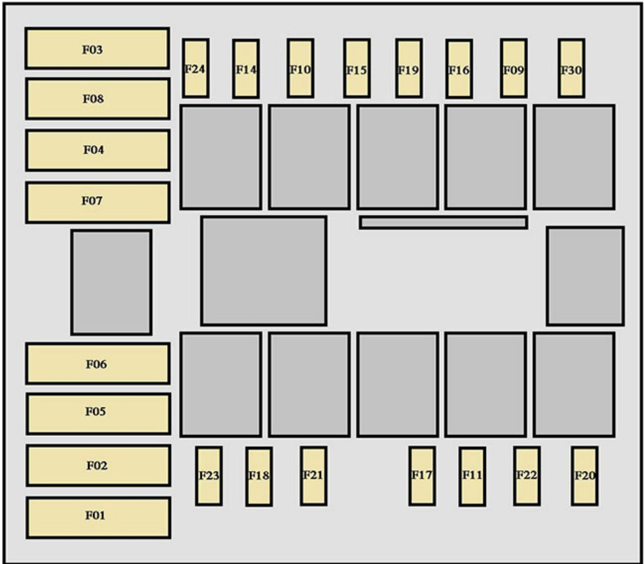
**Assignment of the fuses in the engine compartment (2011)**
