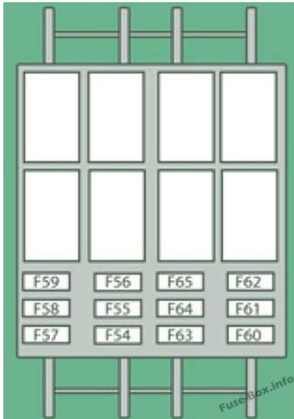
**Assignment of the fuses in the door pillar fuse box (2008, 2009, 2010)**
